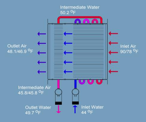
In this example the hot/humid inlet air is cooled with incoming 44 degree water to a fully saturated state at 45.8°F (100% RH). By taking into account the relationship between CFM and GPM the coil was sized such that the leaving water temperature was higher than the air temperature leaving the cooling core. The warmer water is then routed through a re-heat core to increase the air temperature. The result is leaving air that has been de-saturated having a relative humidity of 92 percent.
